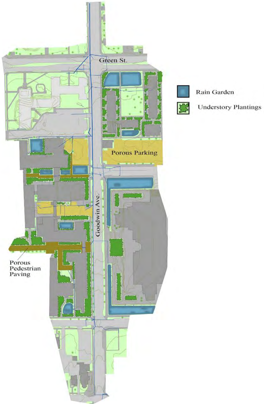
Figure 17: Possible locations of rain gardens, understory plantings, and porous paving around the study area.
