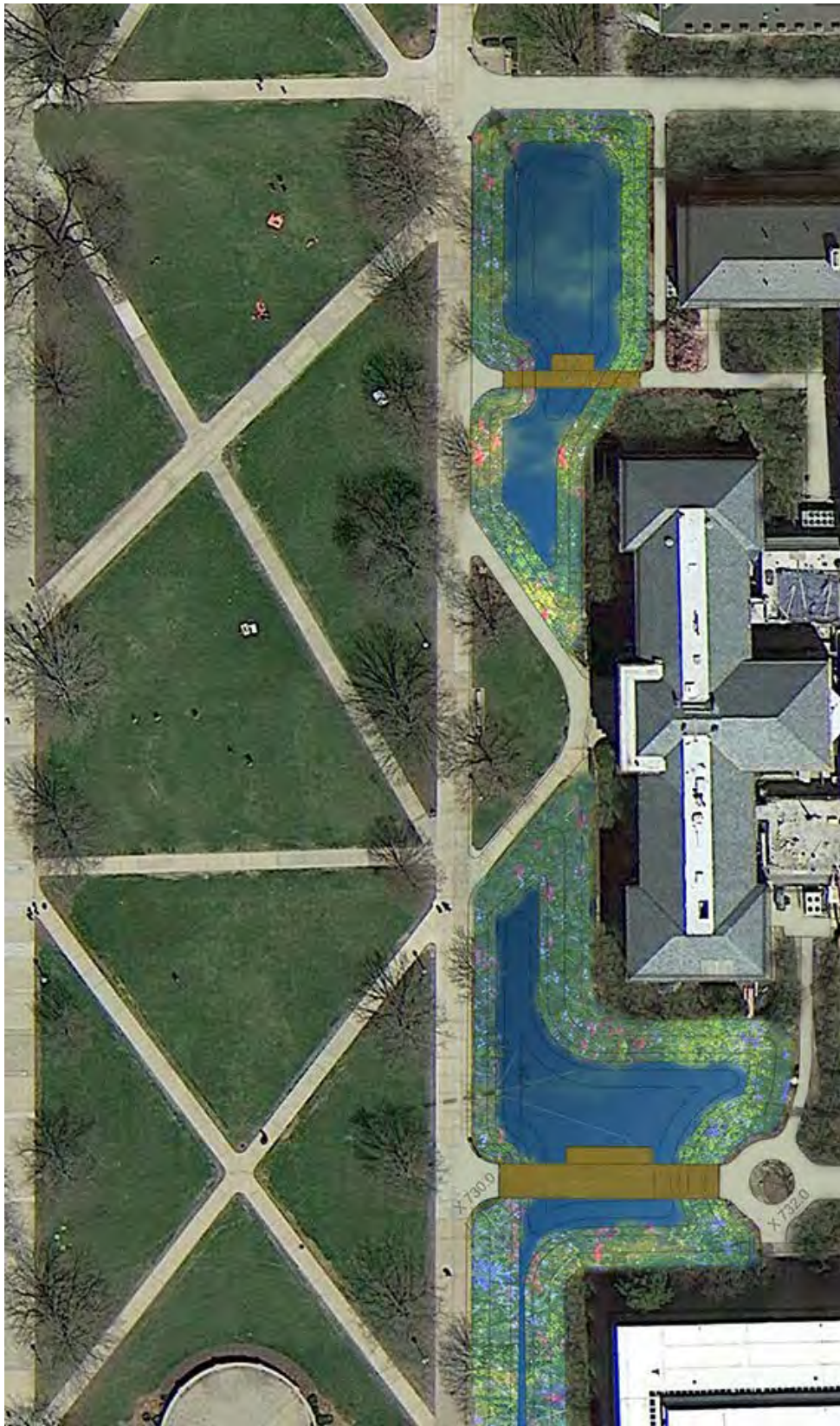
Figure 15: Bio-retention areas around the main quad, in front of Davenport Hall. Bridges across the water would introduce a new pedestrian experience to the campus.
