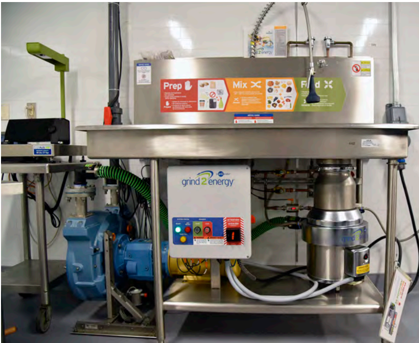
Above: The Grind2Energy system collects food waste from university dining halls so that it can be transported to the Urbana-Champaign Sanitary District and converted into energy. Below: A new, state-of-the-art baler machine was installed at the Waste Transfer Station in 2024 to enhance campus-wide recycling efficiency.
