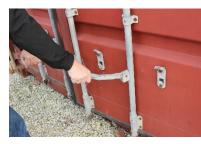
Rotating the levers unlatches the locking pins at the top and bottom of the door.
