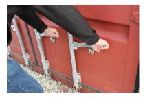
2. Once you have unlatched the levers on one door, rotate the levers toward you until they are at a 90degree angle to the door. Now you can let go of the top pieces, even if they fall back into place.
