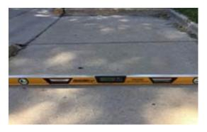
Figure 14 – Curb Ramp Cross Slope
