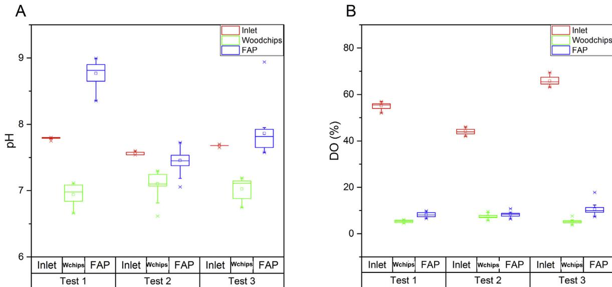
Fig. 4. Each section pH and DO result for all three tests in the box chart (the square in box represents the average and the line is the median).
