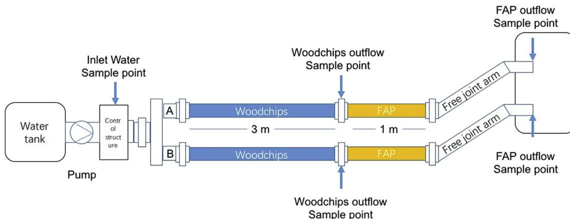
Fig. 1. Illustration of two replicated paired-column configurations using woodchips and fly ash pellets (FAP) fed by a control structure which was supplied water via a pump.
