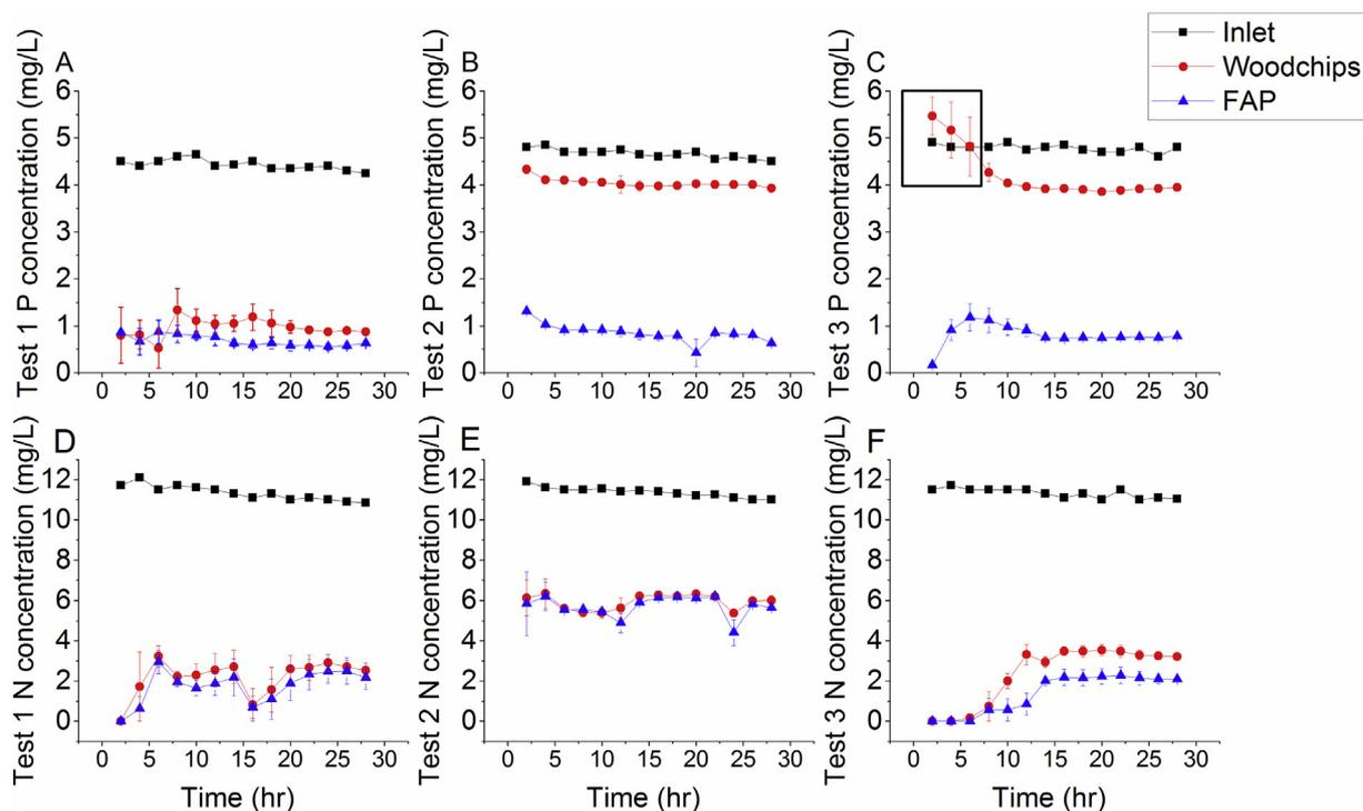
**Fig. 3.** Phosphate (A–C) and nitrate (D–F) concentrations for the inlet, effluent from the woodchips, and effluent from the fly ash pellet (FAP) sections for three tests operated at woodchip section hydraulic retention times of 2.9, 1.5, and 4.2 h (Tests 1, 2, and 3, respectively).
