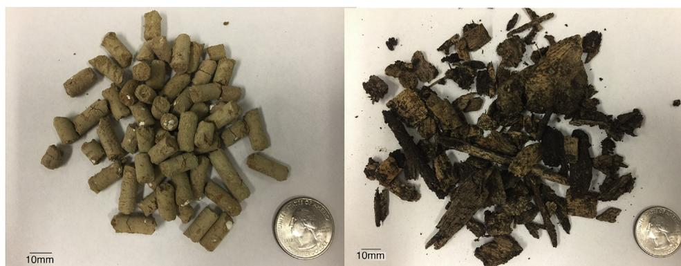
Fig. 2. The fly ash pellets (left) and woodchips (right) used in this study.
