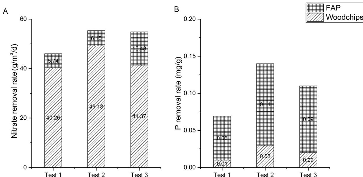
Fig. 5. The nitrate and orthophosphate accumulation removal rate of both sections for all three tests (woodchip section hydraulic retention times of 2.9, 1.5, and 4.2 h, respectively).
