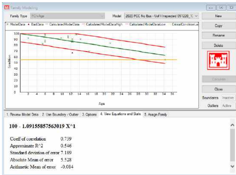
Figure 13. PCC pavement without bus route performance model.
