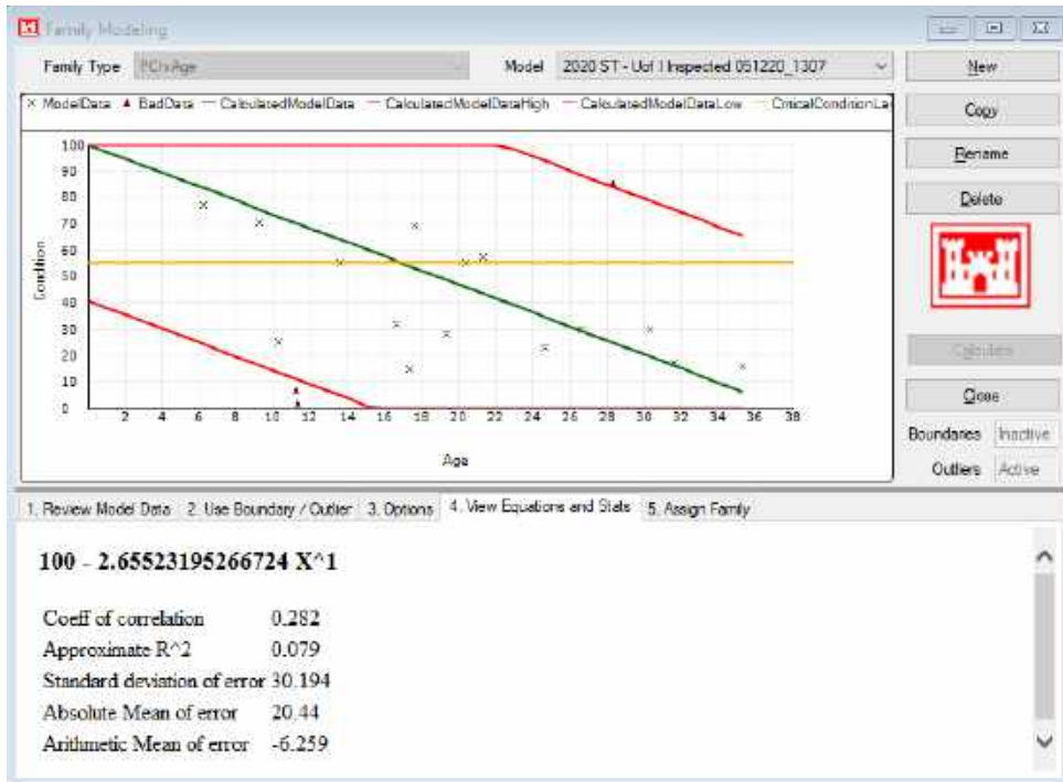
Figure 15. Surface Treatment (oil and chip) pavement performance model.
