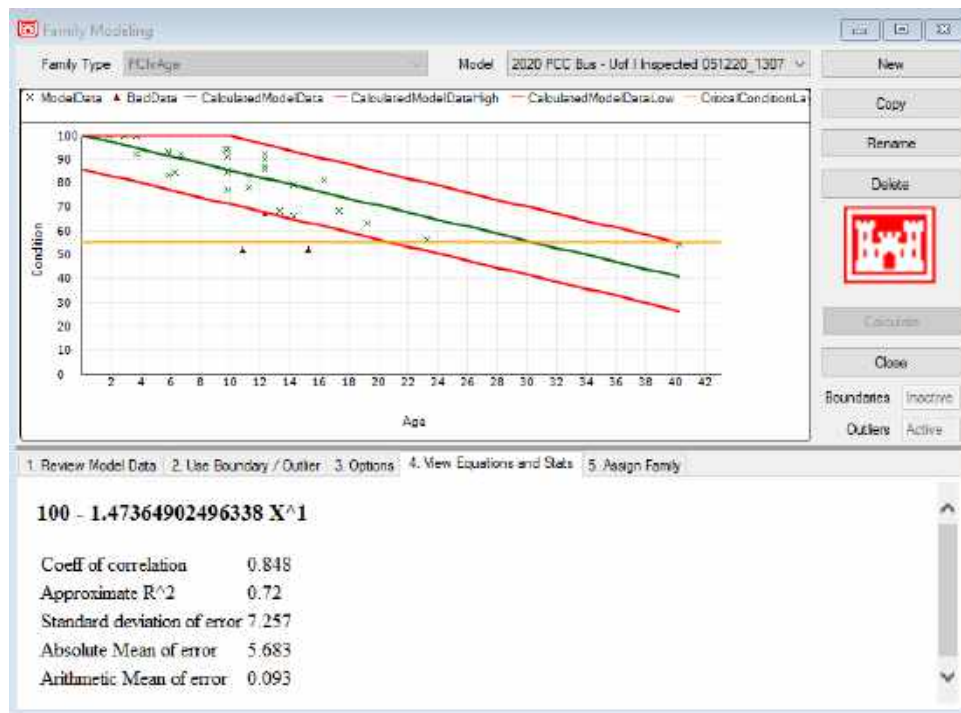
Figure 12. PCC pavement with bus route performance model.
