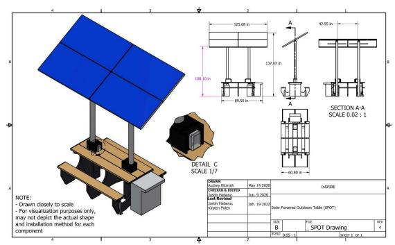
Figure 2.1-1 Overall SPOT Project Structural Design (same as Figure 1.2-1)
