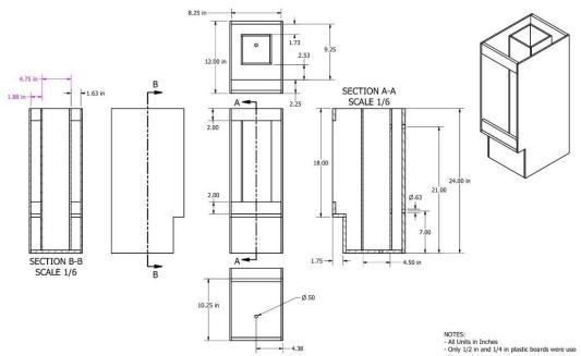
Figure 4.2.3-2 Pole Base Shell Dimensions
