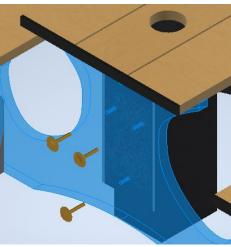
**Figure 4.3.3-2** Close up view of location of strike anchors to be installed.
