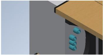
Figure 4.4.4-2 Location of conduit adapters underneath electrical box
