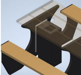
Figure 4.3.3-3 Construction adhesive on pole base
