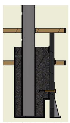
Figure 4.3.4-5 Cut view of pole installation
