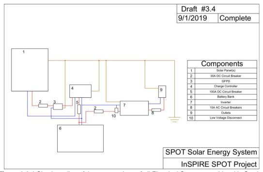
**Figure 3.2-1** Simple outline of the connections of all Electrical Components Listed in Section 3.1. Excluding the temperature control system.
