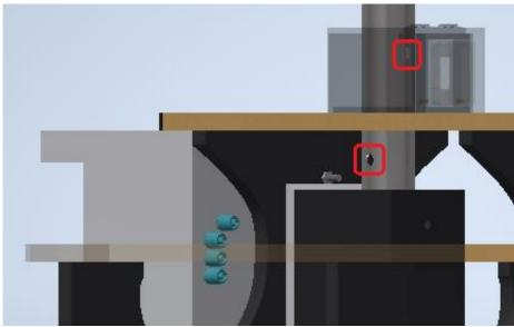
**Figure 4.4.5.3-1** Close up view of underneath the table, location of holes on pole are indicated in red
