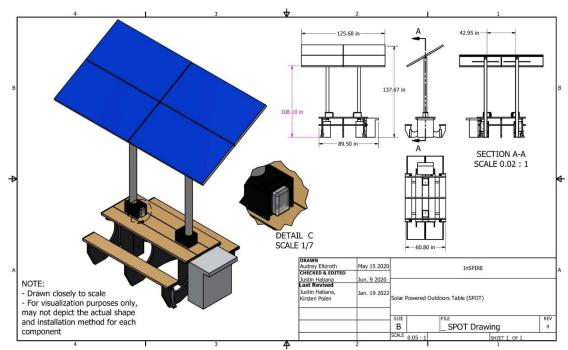
Figure 1.2-1 Overall SPOT Project Structural Design (see attachment A for larger version
