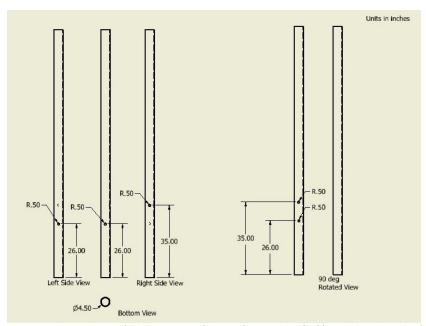
Figure 4.2.4-1 Location of Holes on 10ft long front pole (left) and back pole (right).
