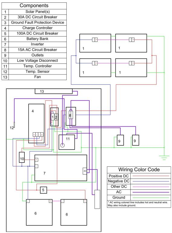
Figure 3.2-2 Model of physical layout of PV system wiring
