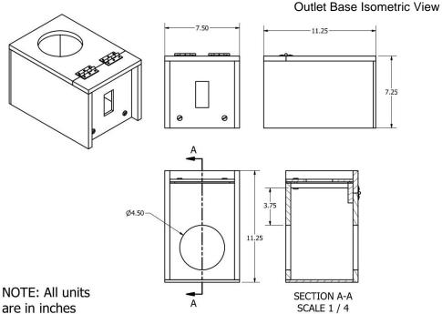
Figure 4.2.2-3 Outlet Base Dimensions
