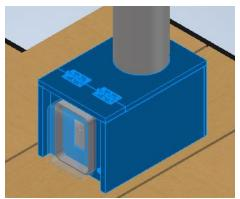
**Figure 4.4.2-1** Installed Outlet Base. Highlighted to show components
