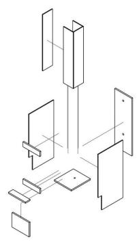
Figure 4.2.3-4 Pole Base Shell Exploded View
