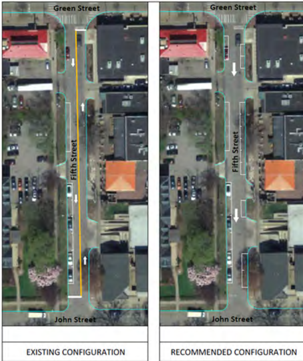
Figure 4.12: Existing and Proposed Lane Configurations for Fifth Street South of Green Street
