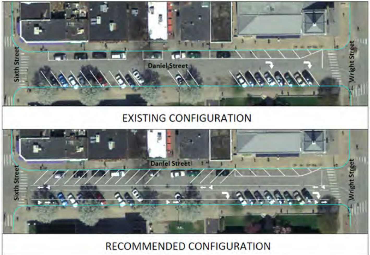
Figure 4.8: Existing and Proposed Lane Configurations for the 600 block of East Daniel Street
