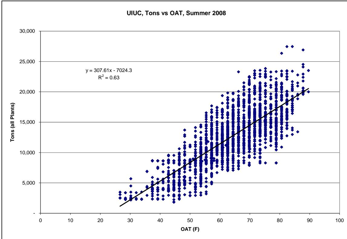
**Figure 3.1-8. Chilled Water Demand (Tons) vs. Outside Air Temperature**
