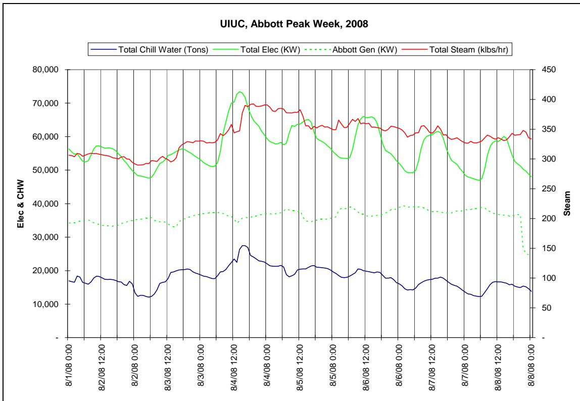
**Figure 3.1-5. Electric, Steam, and Chilled Water Load Profiles –August 1 -8, 2008**
