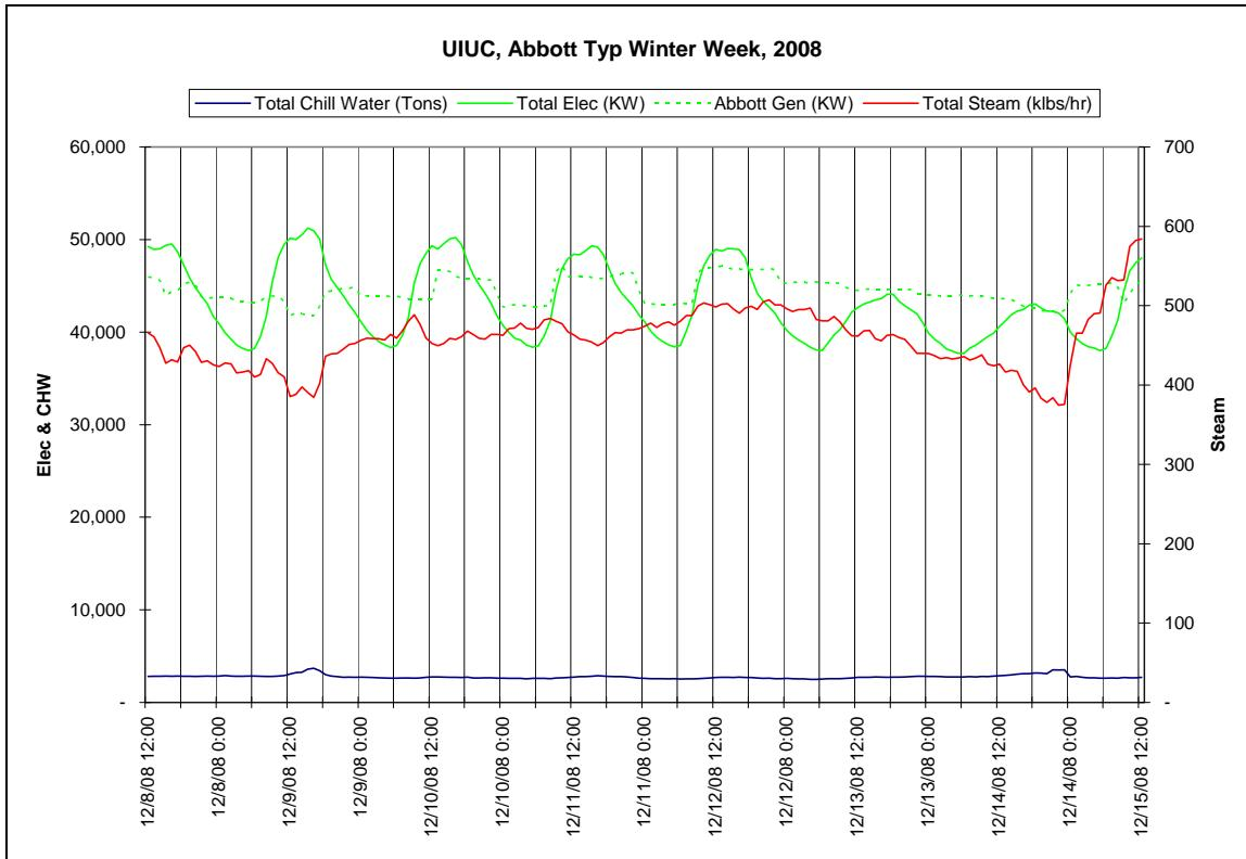
**Figure 3.1-6. Electric, Steam, and Chilled Water Load Profiles – Dec. 8-15, 2008**
