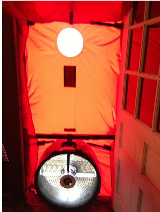
Blower door test in operation
