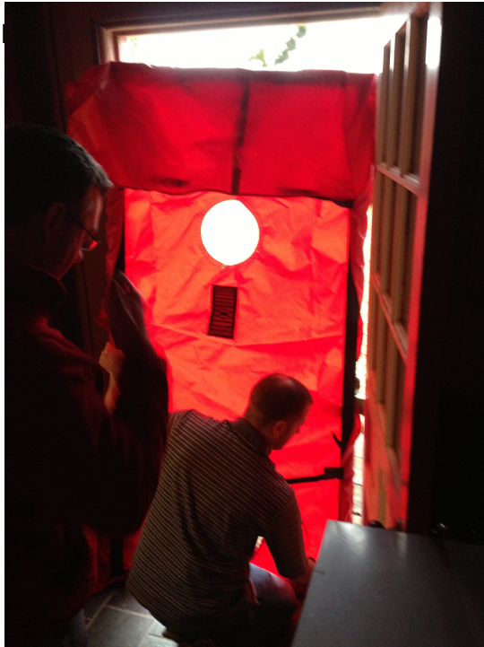
Blower door setup at Gatehouse site
