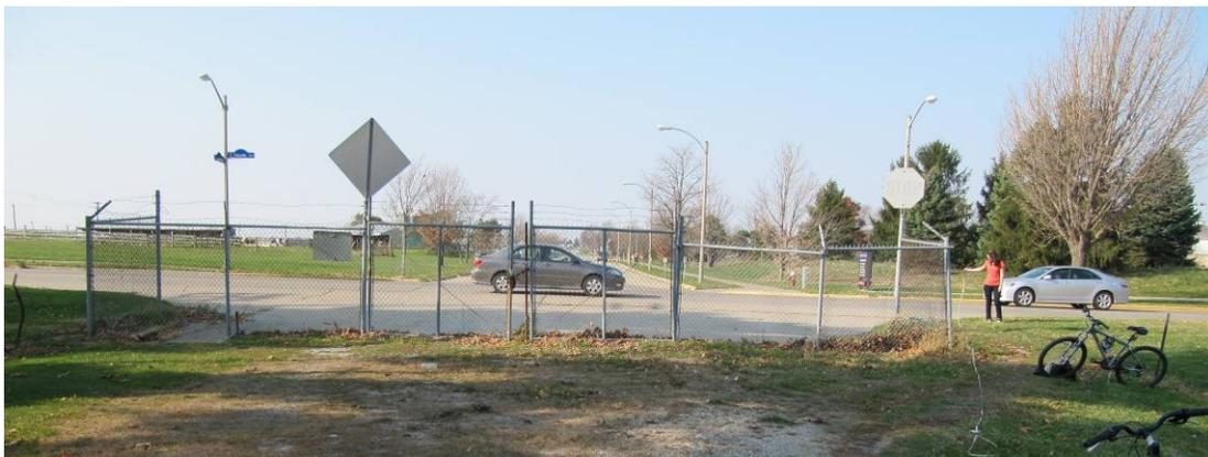
3. Vet Med Gate and Barricade (*below*). At this location, there is a barricade to modify, new gravel to lay, and a fence to modify. The end of street warning barricade will need to be replaced with a barricade that has a five foot opening for bicyclists to pass through. The fence will need to have a section opened up as well, and new gravel will need to be laid from the edge of the pavement on the east to the beginning of the gravel on the west.
