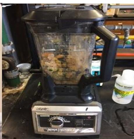
Fig.2 Homogenization using blender
