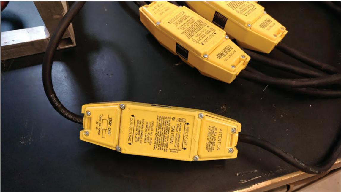
**Figure 7** A Southwire Company circuit interrupter with a 120VAC (volts alternating current) voltage rating, labeled I in Figure 2.
