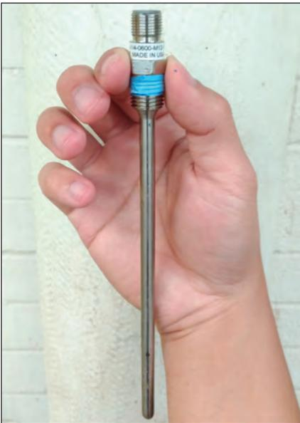
**Figure 4** The PT100 precision temperature sensor shown in Figure 3.
