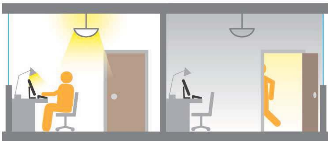
Figure 5: Occupancy sensor & task lighting schematic
