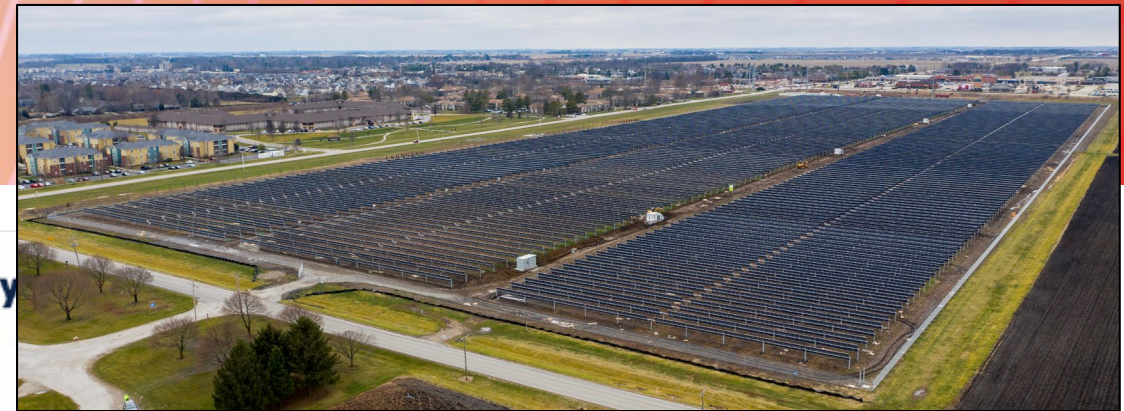
Solar Farm 2.0 (12 MW → 20,000 MWh/yr)
