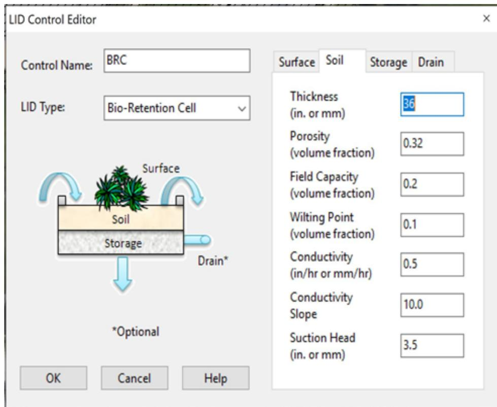
**Figure 4.27** Bioretention swales modeling on EPA SWMM window using LID Controls provision
