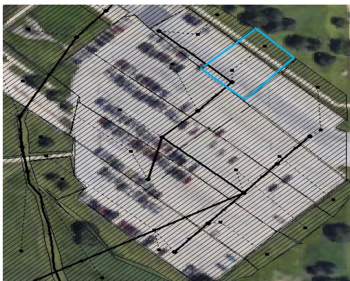
**Figure 4.21** Delineated subcatchment on EPA SWMM window
