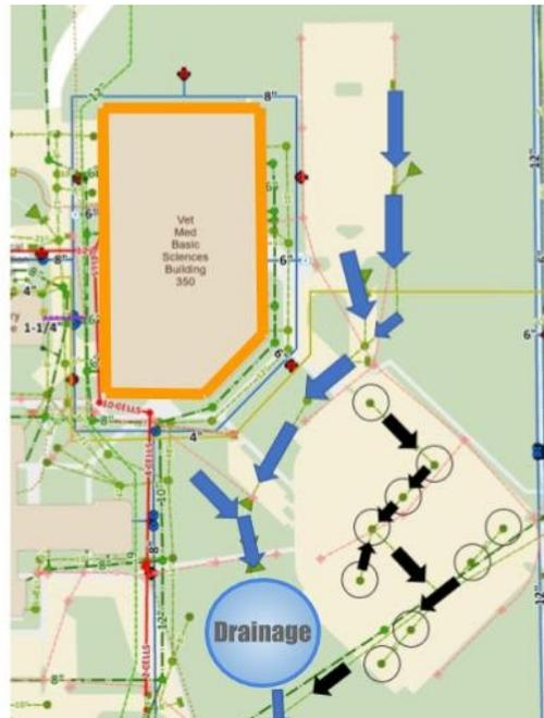
**Figure 1.12** Stormwater routing near entrance to College of Vet Med
