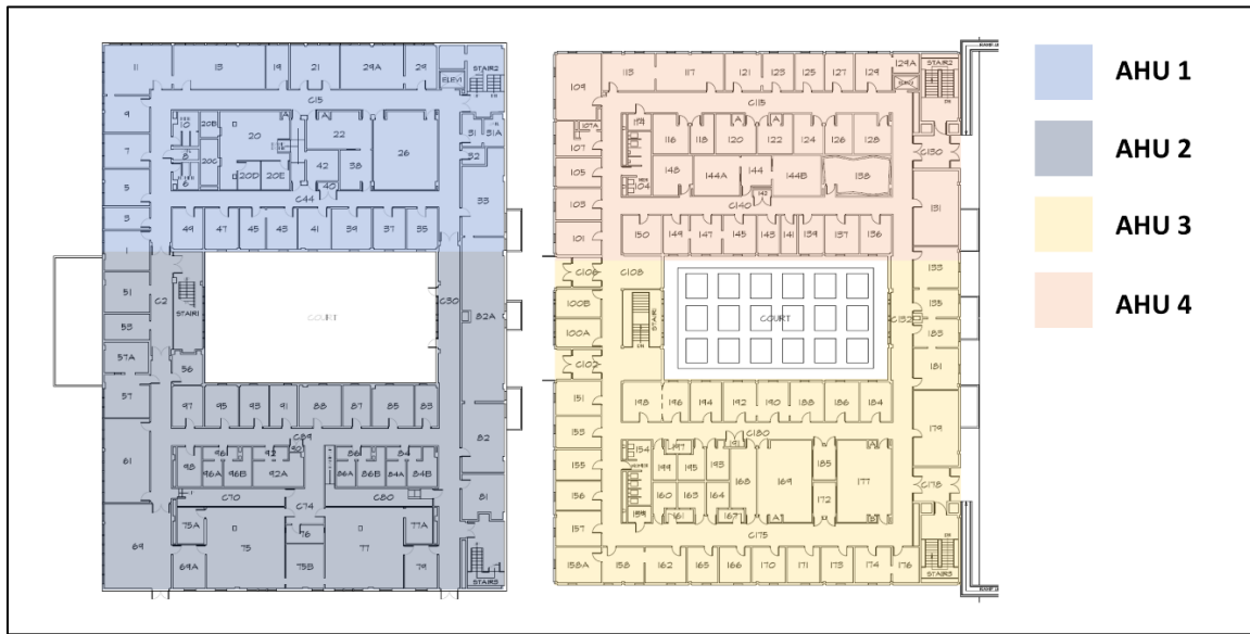
Figure 4 HVAC system zoning
