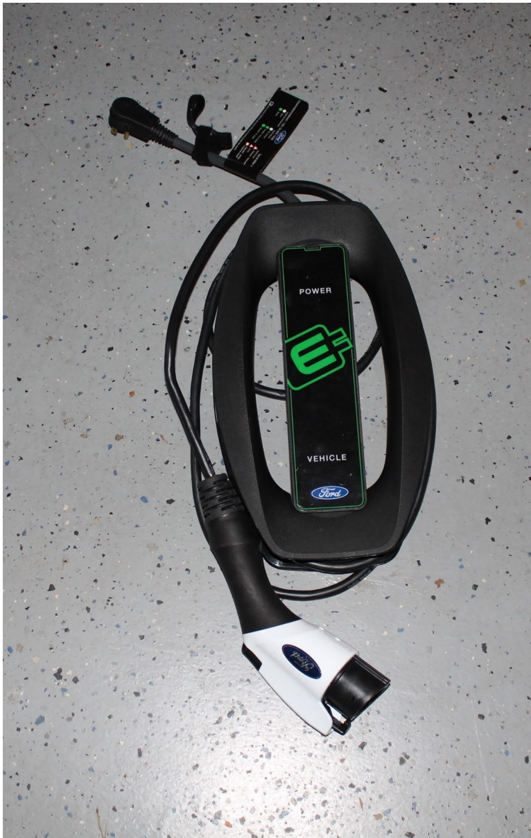
Typical vehicle accessory cable for Level 1 charging.
