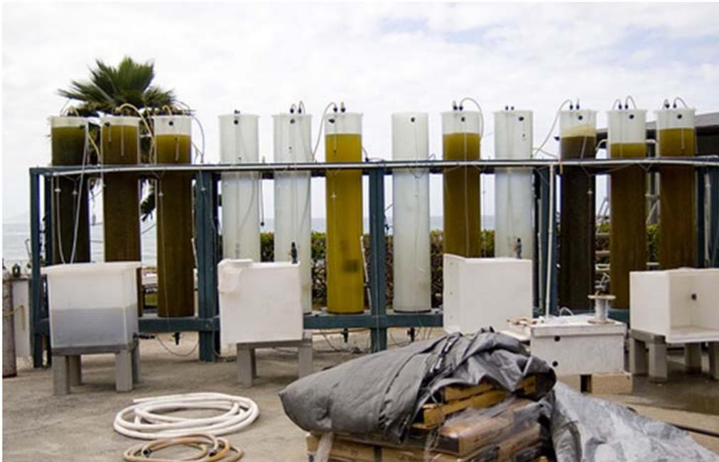
**Figure 2.** Example of outdoor bioreactors used at the University of Hawaii.
