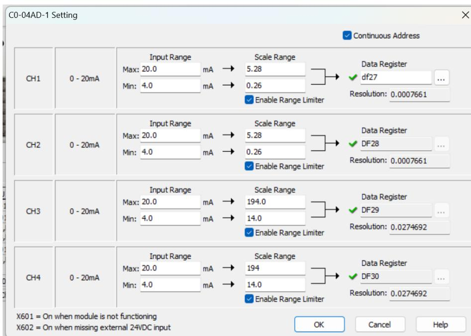
Figure 28. Configuration of Module Inputs (IO6 Flow and Temperature)
