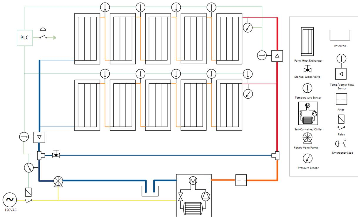
Figure 12. P&ID Schematic of Concept 4
