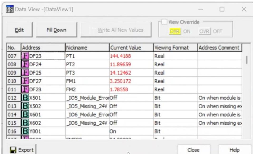
Figure 26. Data Monitor within CLICK PLC Software
