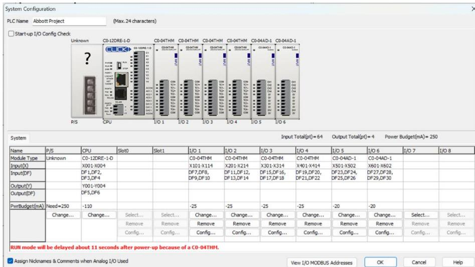
Figure 27. System Configuration for PLC Modules
