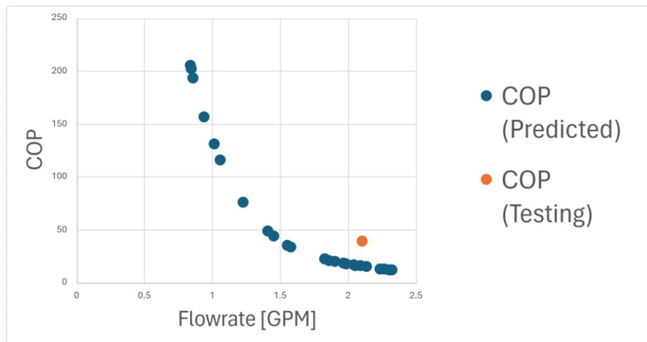
Figure 21. Flow Rate versus Coefficient of Performance for Assembled Panel Array
