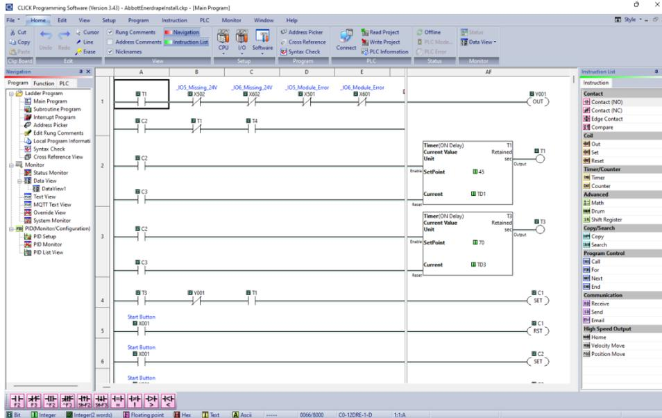
Figure 25. CLICK PLC Software Main Screen
