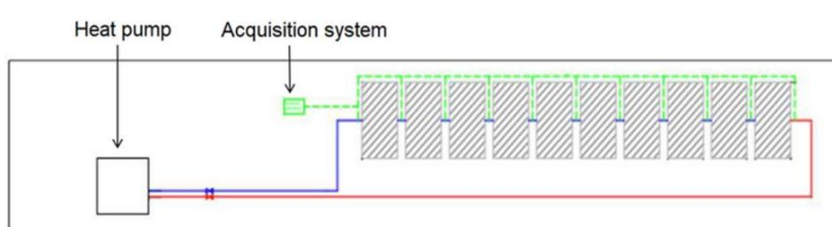
Figure 2. 10 Enerdrape panels connected in series
