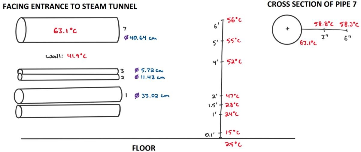
Figure 5. Site Visit Temperature Measurements and Dimensions
