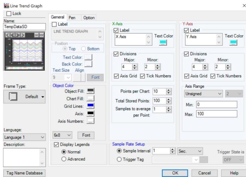
Figure 22. Configuration for Data Storage through C-more Program
