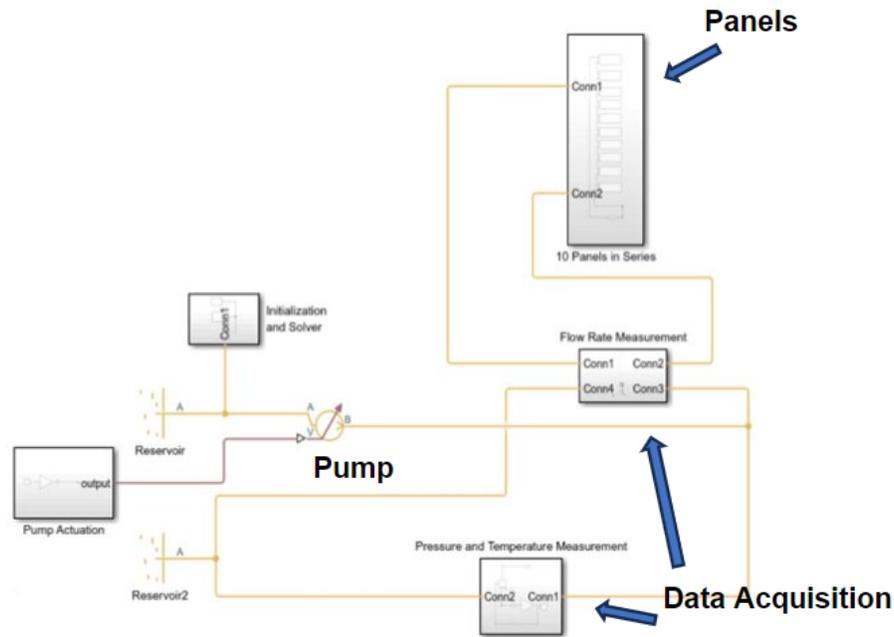
Figure 13. Model of Enerdrape Test Case
