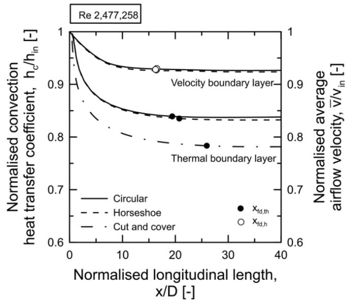
Figure 7. Development of Thermal and Velocity Boundary Layers for Different Cross-Sections [1]
