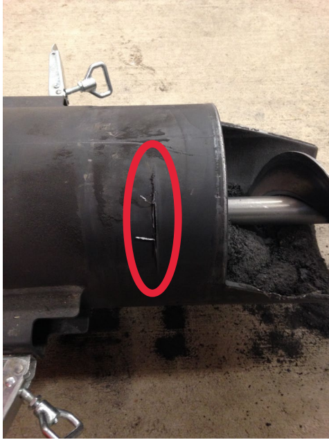
Original cross auger with wear
